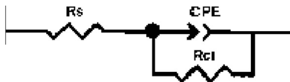
Figure 5 Equivalent circuit model for iron/1.0 M HCl interface.
